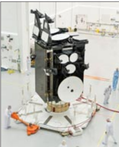
Lockheed uses air bearings with a powered drive to move the 13,600 lb. AEHF SV2 satellite and transport structure.
