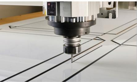
Since a variety of materials are being used for decorative trim, it is important to know what technology to use when manufacturing cladding pieces. Using the right tools minimizes the likelihood for flaws to be created on the routed (or knife cut) piece, even at the very edges. Those flaws can be magnified when a cladding panel is hoisted above a retail shop door or attached to the side of an office building. That means unhappy clients, remakes and scrap, and that's not good for business.
